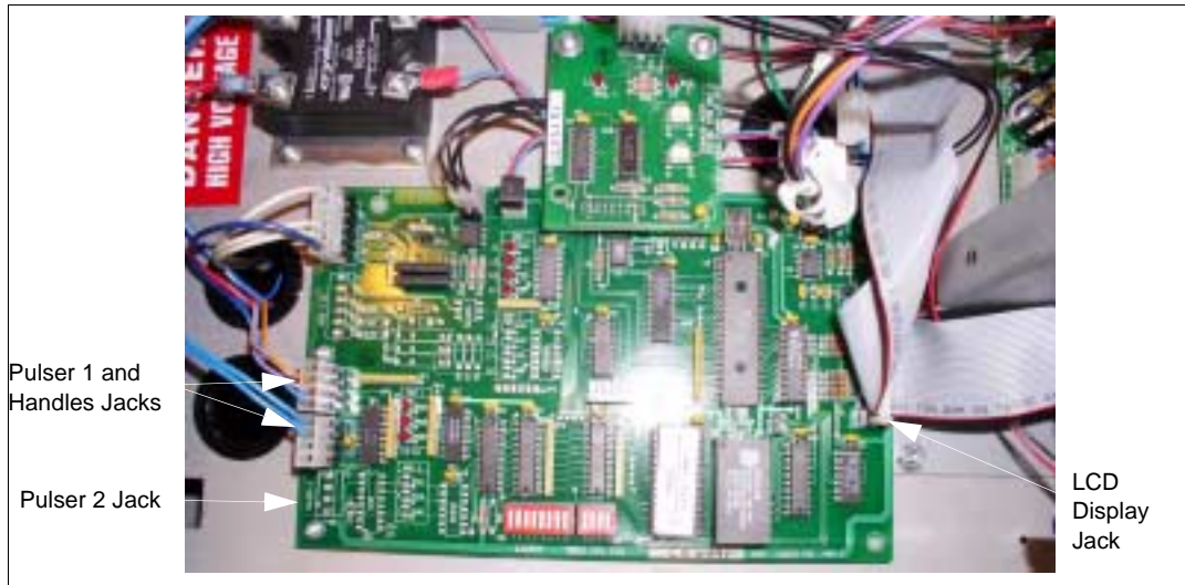
Figure 6: CPU Printed Circuit Board with Original Connections (Picture)
