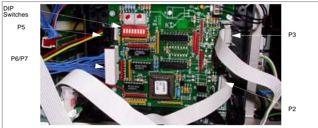
Figure 19: LP-70 Polycase Box Showing Connections
