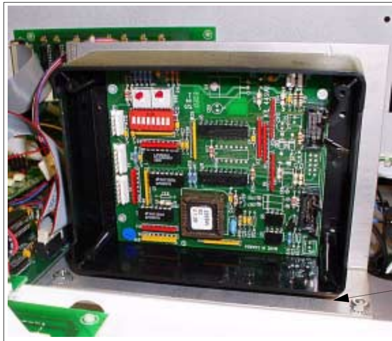
Figure 3: Mounting the LP-70 Polycase Box
