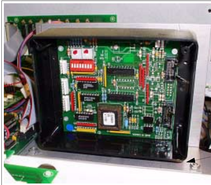
Figure 13: Mounting the LP-70 Polycase Box
