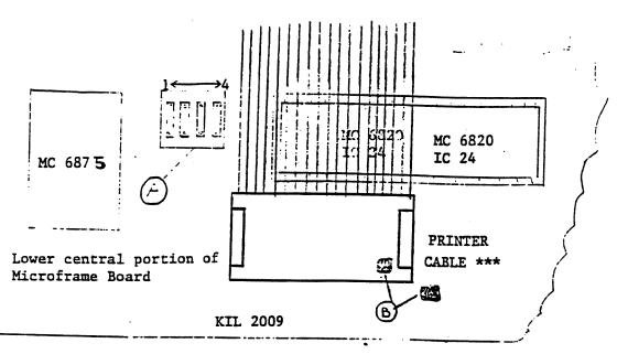
\*\*\* IMPORTANT: REVERSING PRINTER CABLE WILL DESTROY THE PRINTER.
